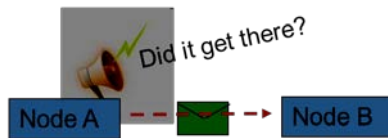
Figure 11. The LLC sub-layer deals with reliable packet transfer.
